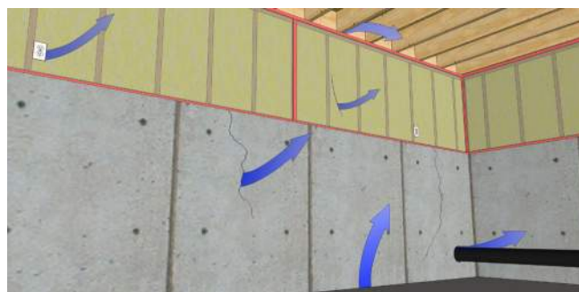
Below-grade wall air sealing locations.
